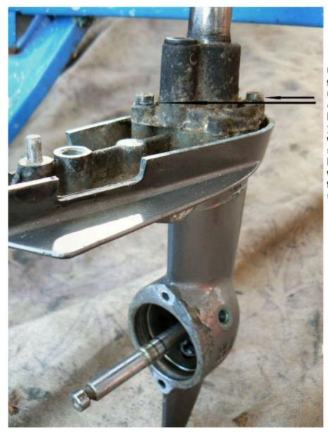
Undo the 2 bolts holding the water pump cover. Gently separate the cover from the base. Note that at this point you will also be withdrawing the driveshaft from the gearbox. Do not lose the cog which will be loose inside the gearbox once the shaft is withdrawn.
