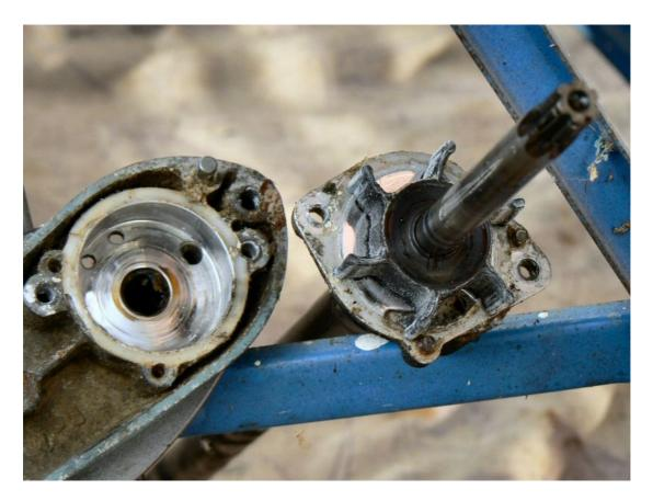
Once separated, the impeller can be slid off the drive shaft. Do not lose the drive pin which is a loose fit into the shaft.
